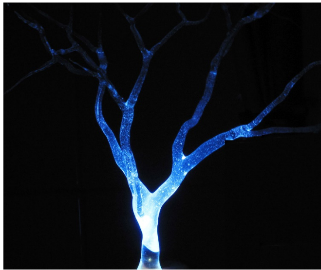
Figure 2 – Result of an experiment made with europium doped borosilicate glass (lampwork); Robert Wiley (2012). In this case a 365nm UV LED was placed under the object.
